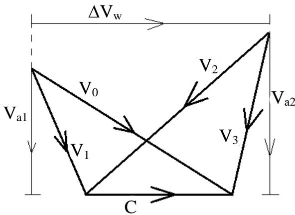
$V_0$  (噴嘴出口速度) =  $290 \text{ (m/s)}$
